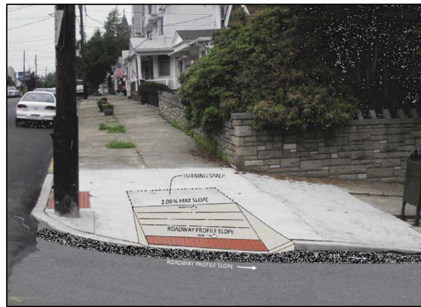
RAMP CROSS SLOPE TRANSITION TO MATCH ROADWAY PROFILE SLOPE
